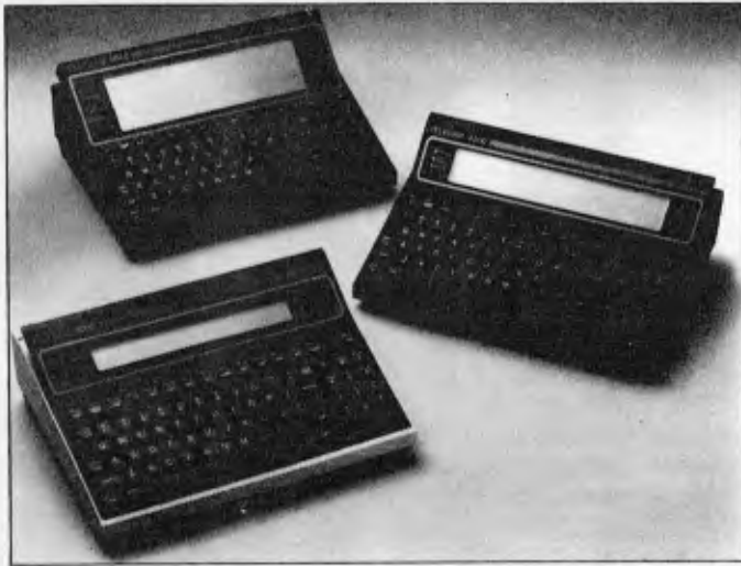
The Teleram range of 16-line LCD micros: the T-5000 8-bit machine costs $2500 and uses the Zilog Z80L and CP/M-80.
